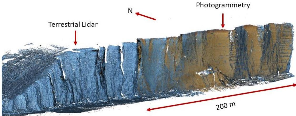
Figure 2: Terrestrial lidar, photogrammetry, and multi-temporal airborne models were used to support learning exercises involving structural and hazard characterization.
