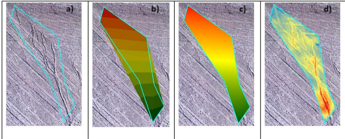
Figure 2: The principle of operation of the tool: a) Polygon of rill boundaries, b) TIN model of rill area and terrain model, c) Smoothed surface model.
