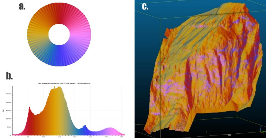
Figure 2: Representation of a diaclosed rock outcrop surface normals. a: Circular CET-C1 color ramp with 4 dominant colours (Kovesi). b: Dip-direction histogram with rotated circular ramp to match the outcrop's principal poles. c: Point cloud of a Swiss cliff with our optimized dip-direction ramp. Two orthogonal planes dominate in dark red and yellow. Pink surfaces correspond to a minor mode made by shallow overhangs.
