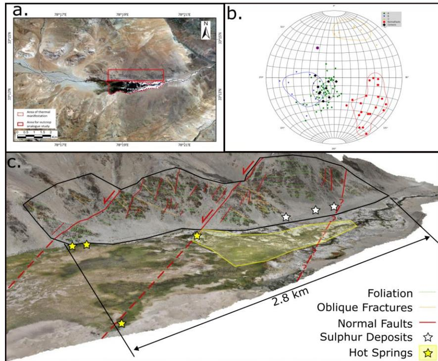
Figure 1: Reservoir analogue outcrop adjacent to the Puga hot springs site (a). Structural measurements (b) extracted from the digital outcrop model (c) have been plotted using a lower-hemisphere stereographic projection, and highlight several sets of fractures and faults that likely controlled fluid circulation prior to their exhumation.
