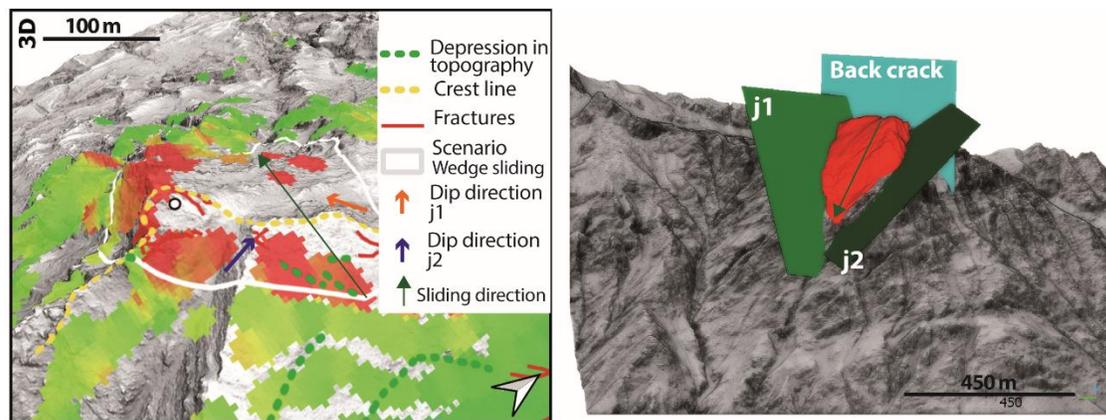
Figure 2: Failure scenario proposed in the case of a wedge sliding structurally constrained by two joint sets  $j_1$  and  $j_2$ . (a) Delimitation of the scenario (b) Planes delimitating the sliding volumes, constructed in Cloud Compare
