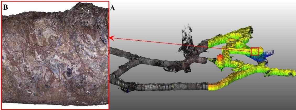
*Figure 1: An example of the reconstructed adit no. 18, A – an overall view of the 3d model; B – a closeup of a 2.5x2.5 m part of the corridor wall.*
