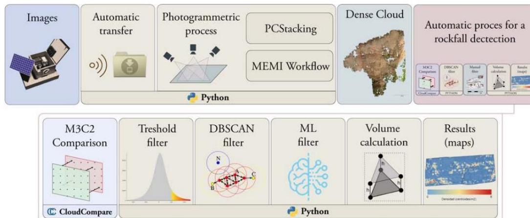
Figure 1: Classic workflow to obtain a change detection comparison from two different point cloud. In this example, the SfM-MVS photogrammetric process (first row) is used to obtain the point clouds
