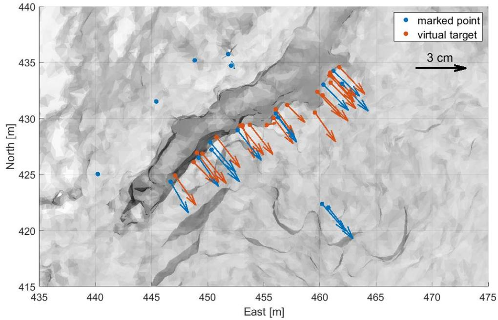
Figure 2: Deformation vectors on Mt. Hochvogel between 2018 and 2019.
