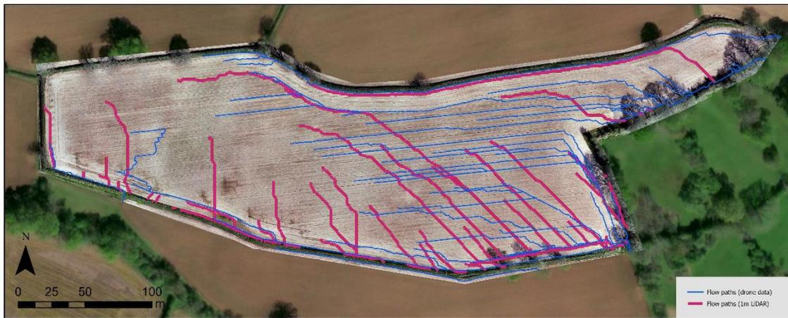
Figure 2. Validation of modelled flow paths in SCALGO Live (<https://scalgo.com/>) between EA 1m LiDAR data (pink) and 1.84cm/pix resolution drone data from DJI Phantom 4 RTK (blue) in Herefordshire, UK. The drone orthophoto is overlaid on the base map sourced from Mapbox (SCALGO Live 2023).
