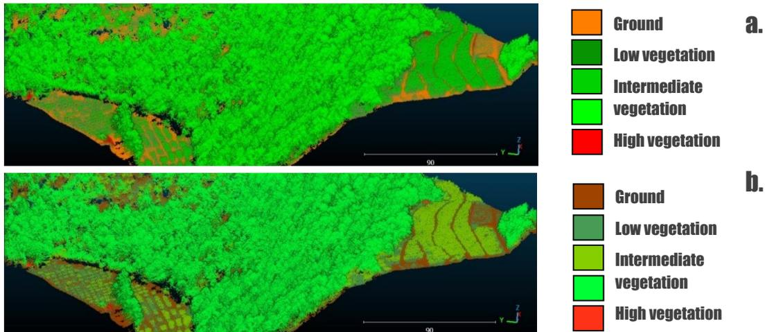
Figure 1: Representation of classes using discrete colours of a countryside landscape close to Sion (Switzerland). a: colours from an industrial standard (TerraScan). b: our colour ramp improves visual class contrasts (at least 40 CIELab space units) and lightness ordering is coherent with above-ground elevation (lighter is higher).
