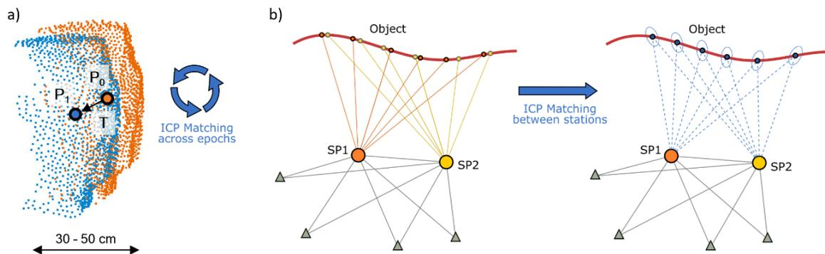
Figure 1: a) Creation of corresponding virtual targets using ICP matching and b) integration into the geodetic monitoring network.
