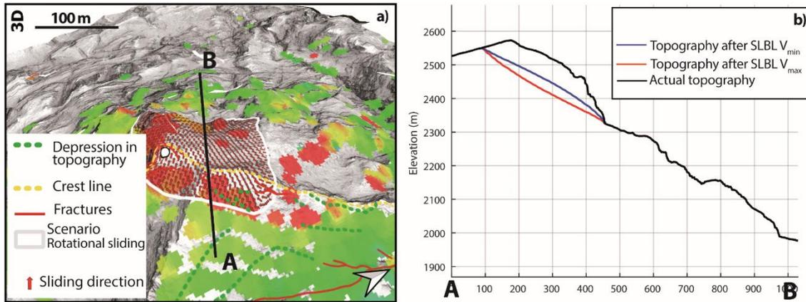
Figure 1: Failure scenario proposed in the case of a rotational sliding defined by SLBL. (a) Delimitation of the scenario and sliding direction (b) Profile of the sliding base level
