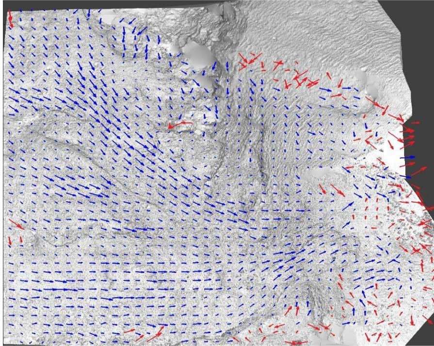
Figure 1: The red arrows indicate the displacements that are considered outliers based on histogram analysis.
