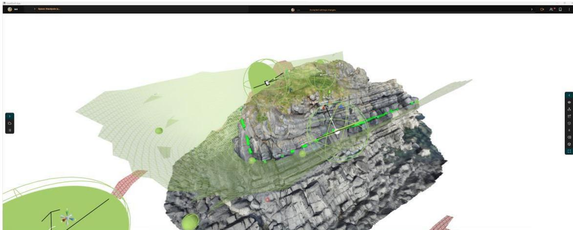
*Figure 1 Screenshot from the LiquidEarth platform showcasing the interpretation of an outcrop. The image highlights the application's capability to create and modify 3D geological models in an immersive mixed-reality environment*
