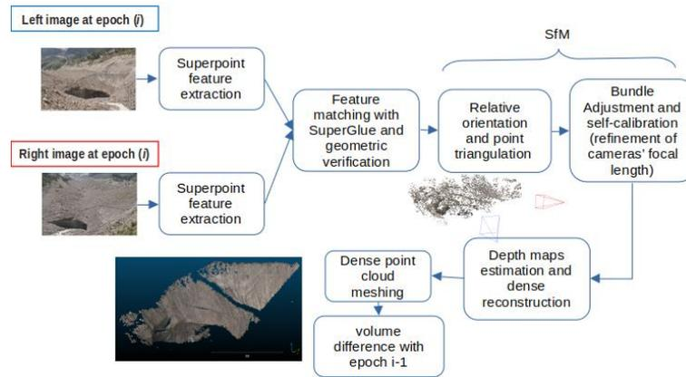
Figure 1. Scheme of the main workflow that can be performed with ICEpy4D.
