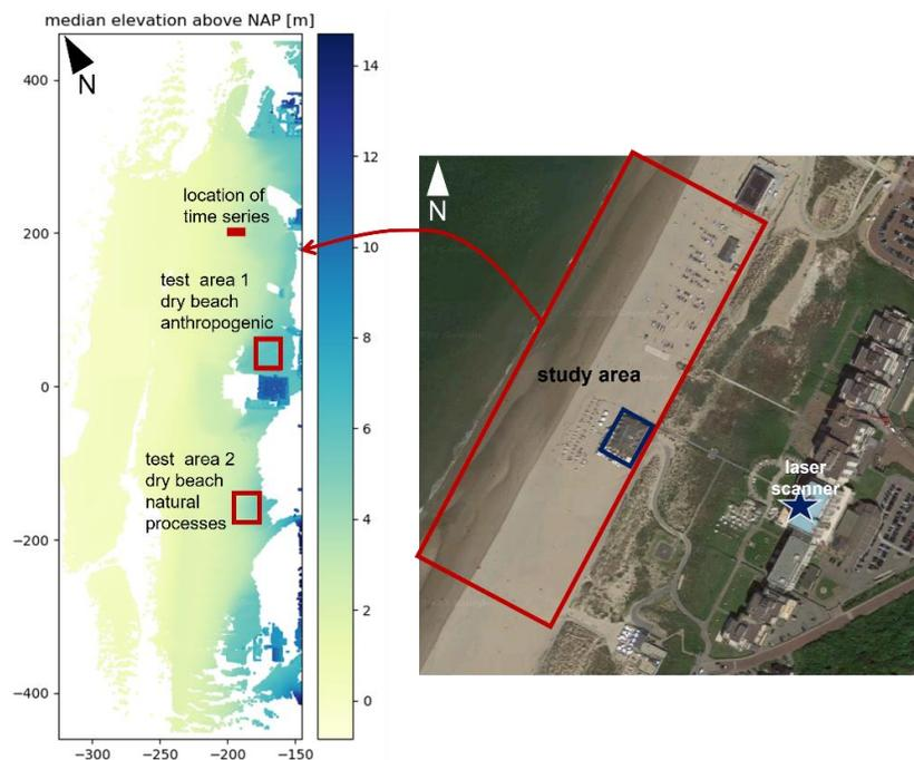
Figure 1: Overview of study site with aerial image (© Googlemaps) and point cloud of the beach area colored according to elevation. Two test areas are marked with red squares and the location of the time series in Figure 2 are indicated with a red bar.
