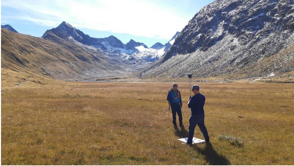
*Figure 1: Measuring targets in the field for georeferencing 3d point clouds and orthophotos from photogrammetric unteamed aerial vehicle surveys.*
