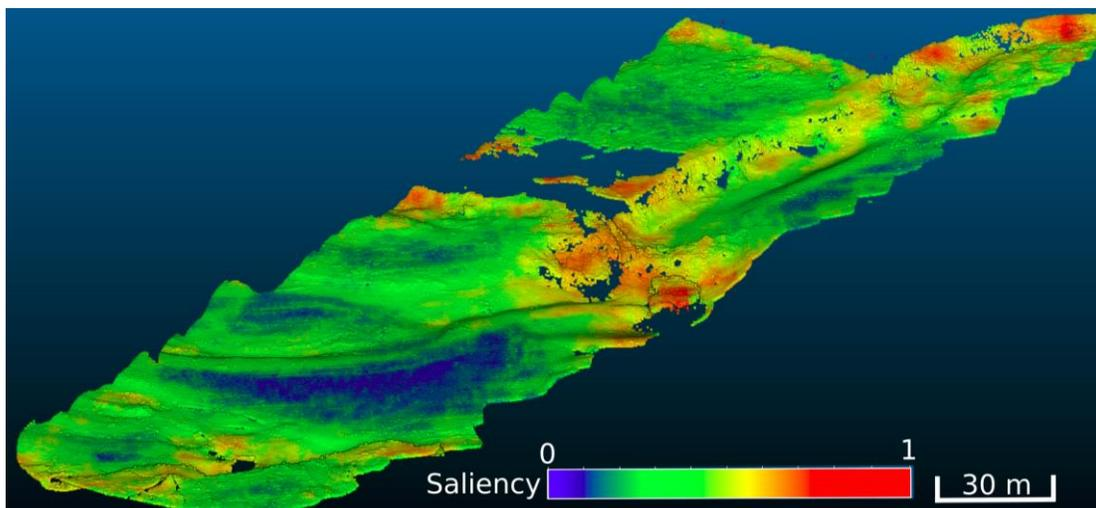
Figure 1: An extract of saliency evaluation by learning surface reconstruction of a point cloud in the Pielach River (Austria).
