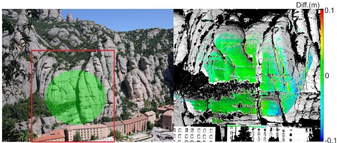
Figure 2: Use example of TLS Avia. Left: Montserrat mountain (Barcelona, Spain) showing the compared area between TLS Iiris-3D and TLS Livox Avia (green circle), the red box frames the image on the right image. Right: Results and scale of the differences.
