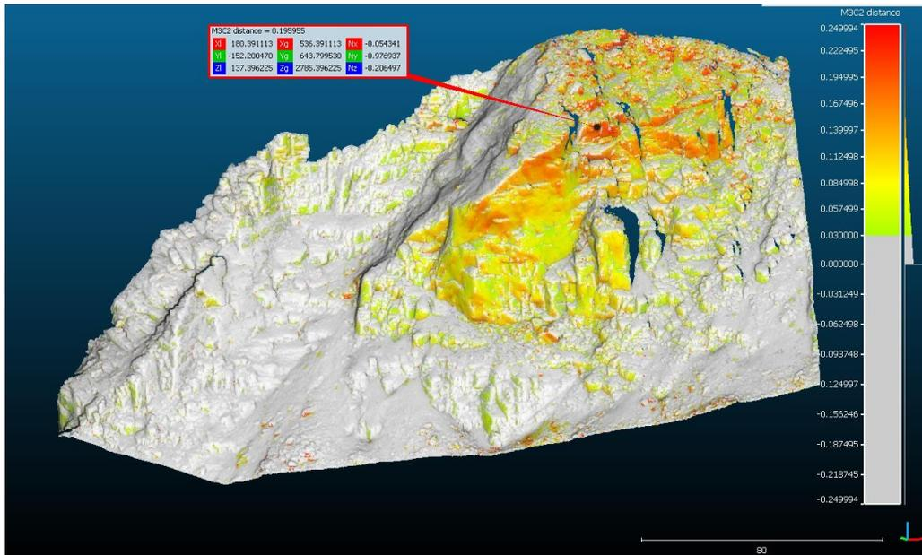
Figure 2: Displacements of the rock face in the summer of 2022, reaching up to 20 cm, as measured by differencing two consecutive laser scans at the beginning and end of the summer.
