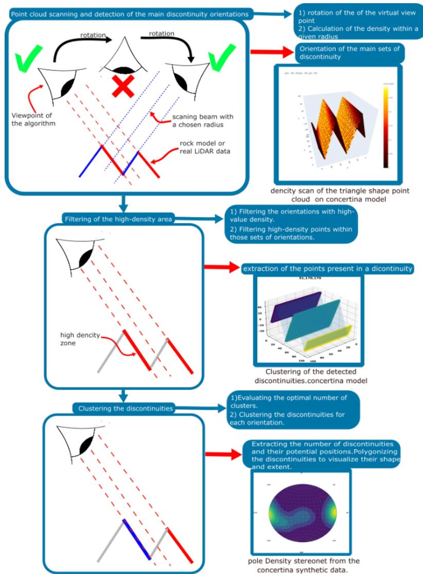
Figure 2: schema describing the 3 main step of the discontinuity detection algorithm.
