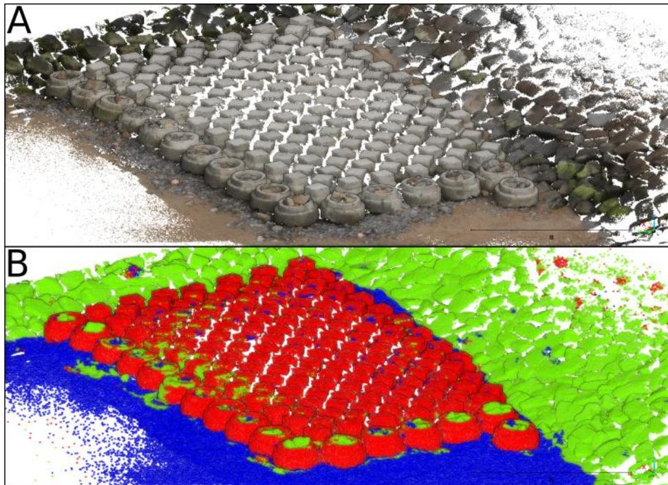
Figure 3: A. SfM point cloud over a coastal dike;
