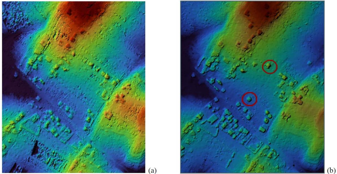
Figure 1: Zoom-in of the derived DEM from Pleiade images, acquired in (a) 2015 and (b) 2018, using SfM-MVS.
